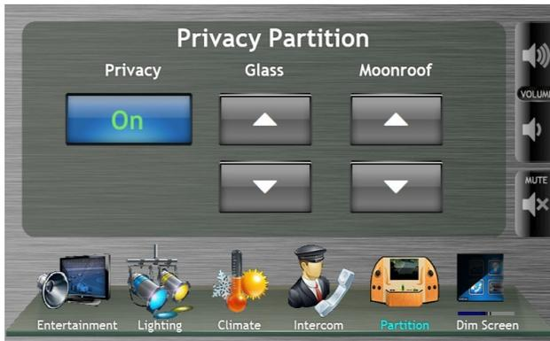
Figure 12: Layout B,C,and D: Privacy On/Off, Glass Up/Down, Moonroof Open/Close
