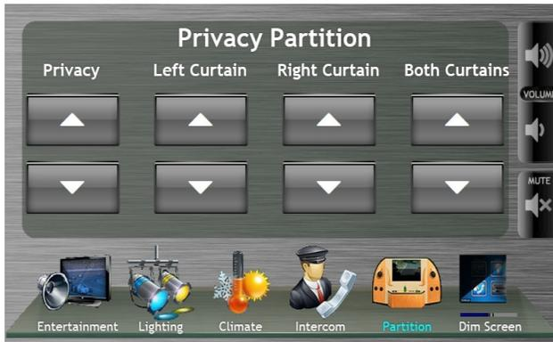
Figure 15: Layout A,E,F,G: Privacy Up/Down, Left,Right,and Both Curtains Up/Down
