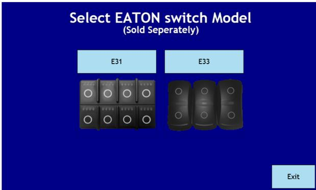
External switch panels are now available. The switches work in parallel with the touchscreens. They provide an 'Always Available' switch options.
