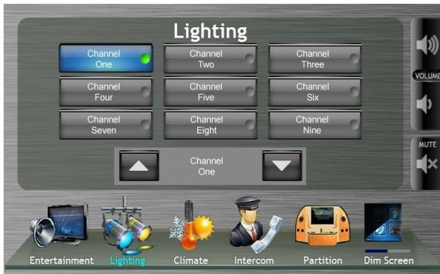
In order to control a lighting channel, the channel must first be selected. The selected lighting channel will have a blue background, and the control box at the bottom will show the selected channel name.
