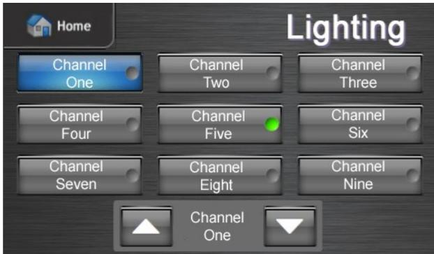
To control a light, the channel must first be selected. When a channel is selected, the background turns blue, and the Channel name appears in the lower control box. In this example, Channel One is selected. If a channel is On, a Green Indicator will appear. In this example, Channel Five is On and all the others are off.
