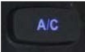
**A/C** – When you press this button it will activate the A/C and turn on the blower motors to low speed. Pressing the button again will increase the fan speed in steps up to the maximum, and then back to off.
