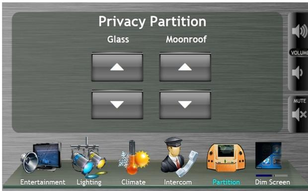
Figure 11: Layout C and D: Glass Up/Down and Moonroof Open/Close
