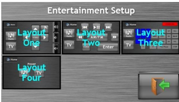
Select the layout that matches the one selected on the Passenger screen. The passenger screen controls the Universal Infrared Remote Control transmitter, if installed.
