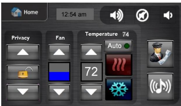
The In-Motion screen allows you to quickly control most of the features directly from one screen. Use the 'Home' button to see all of the control options. Depending on which options are installed in the vehicle, some of the controls may be hidden.
