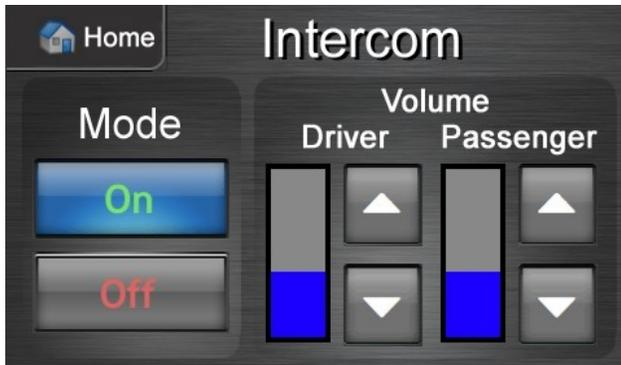
The intercom can be turned on and off from this screen. The Driver's Volume and the Passenger's Volume can be adjusted independently. Passengers also have the ability to adjust the Passenger Volume from the rear screen. If your vehicle is not equipped with an intercom, this page will be hidden.
