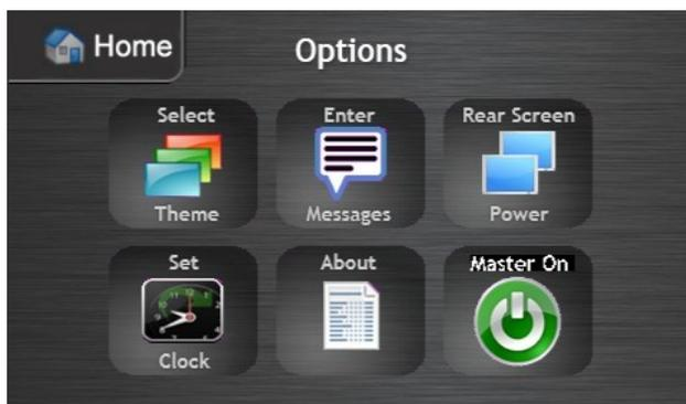
From the Driver's Options screen, you can select a Theme to be displayed on the Passenger's screen. You can also enter a four line message that is displayed on the Passenger screen. To turn the System On or Off, press and hold the Master button.
