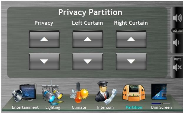
Figure 13: Layout A, E, and F: Privacy Up/Down, Left & Right Curtains Up/Down
