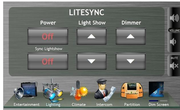
The Litesync module can be turned On or off from this screen. To change the pattern of the selected light show, use the Light Show Up and Down buttons. To increase or decrease the brightness of the RGB lights, use the Dimmer Up and Down buttons.
