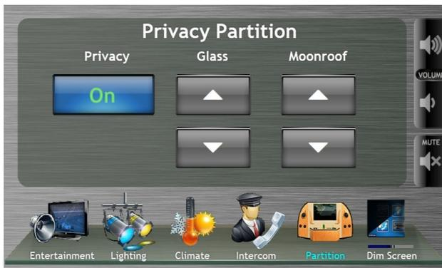
Figure 20: Layout B,C,and D: Privacy On/Off, Glass Up/Down, Moonroof Open/Close
