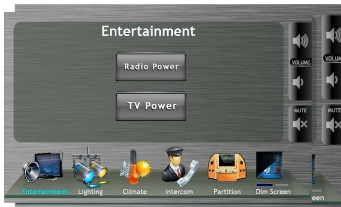
The 'Power' buttons will turn the TV or Radio On or Off. If the power is on, the power button will be blue. If the power is off, the power button will be gray. The other buttons operate the Universal Remote Control function.
