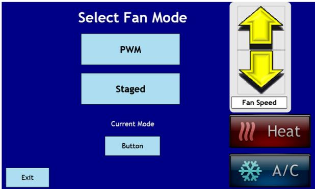
For both PWM and Staged modes, different fan outputs can be selected for when the AC is on, the Heat is on, or only the Fan is on.
