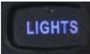
**Lights** – When you press this button, it will turn on all of the lighting controlled by the Smarttouch system to full brightness. Pressing a second time will turn all of the lights off.
