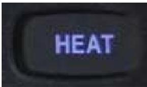
**Heat** – When you press this button it will activate the Heat and turn on the blower motors to low speed. Pressing the button again will increase the fan speed in steps up to the maximum, and then back to off.
