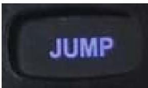
**Jump** – When you press this button it will activate the Jumpstart Solenoid to connect the Main battery to the Auxiliary battery, allowing you to start the vehicle if the Main battery has gone dead. Activating jumpstart will turn off all of the system outputs for several minutes to allow the battery to recharge before being used. This feature will only function if one battery is low, and the other battery is charged. To Activate Jumpstart, press and hold the button. After 5 seconds, the Master
